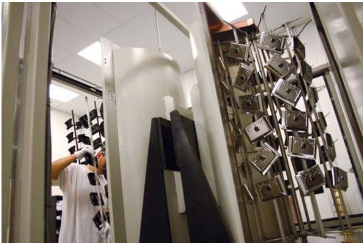
Vacuum metallizing can be used for complex shapes, but often requires a mask to ensure that the metal is deposited in the correct locations. This can be done either by custom mask tooling or by hand masking although custom mask tooling is preferred for larger volumes.
